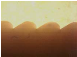
A cross section view of an injection molded Fresnel lens shows poor microstructure replication
