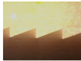
The same view of a Fresnel lens molded by Reflexite shows sharp facets and greatly improved replication
